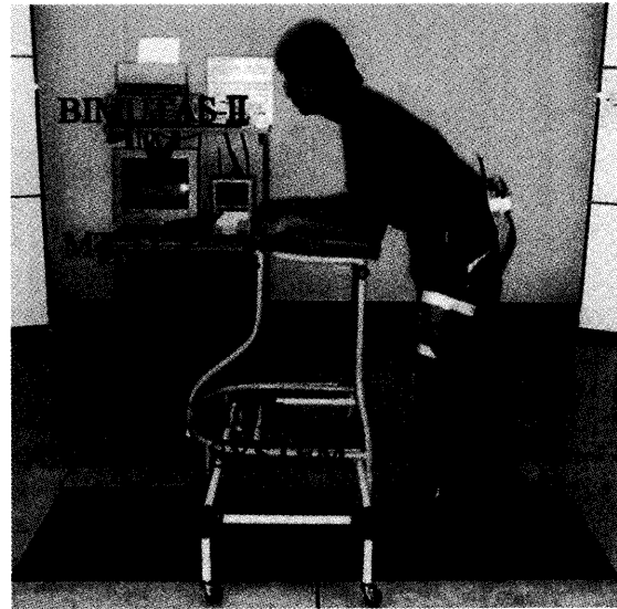
Fig. 2 Determination of the ground reaction force and muscle activation level during the walker gait. The position of the electrodes for the rectus femoris muscle is the middle point of a line which connects the anterior superior iliac spine with the anterior superior margin of the patella. The position of the electrodes for the biceps femoris muscle is the middle point of a line which connects the ischial tuberosity with the head of fibula.
